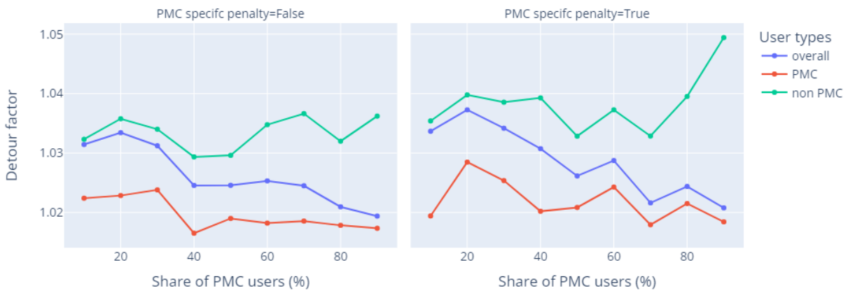
Figure 36: Detour factors in function of the share of PMC users with and without the PMC specific penalty in the HCRS algorithm.
