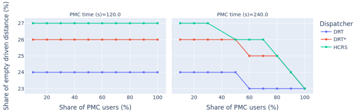
Figure 16: Observed shares of empty driven vehicle distances with a 100 vehicles fleet under various shares of PMC, comparing across algorithms.
