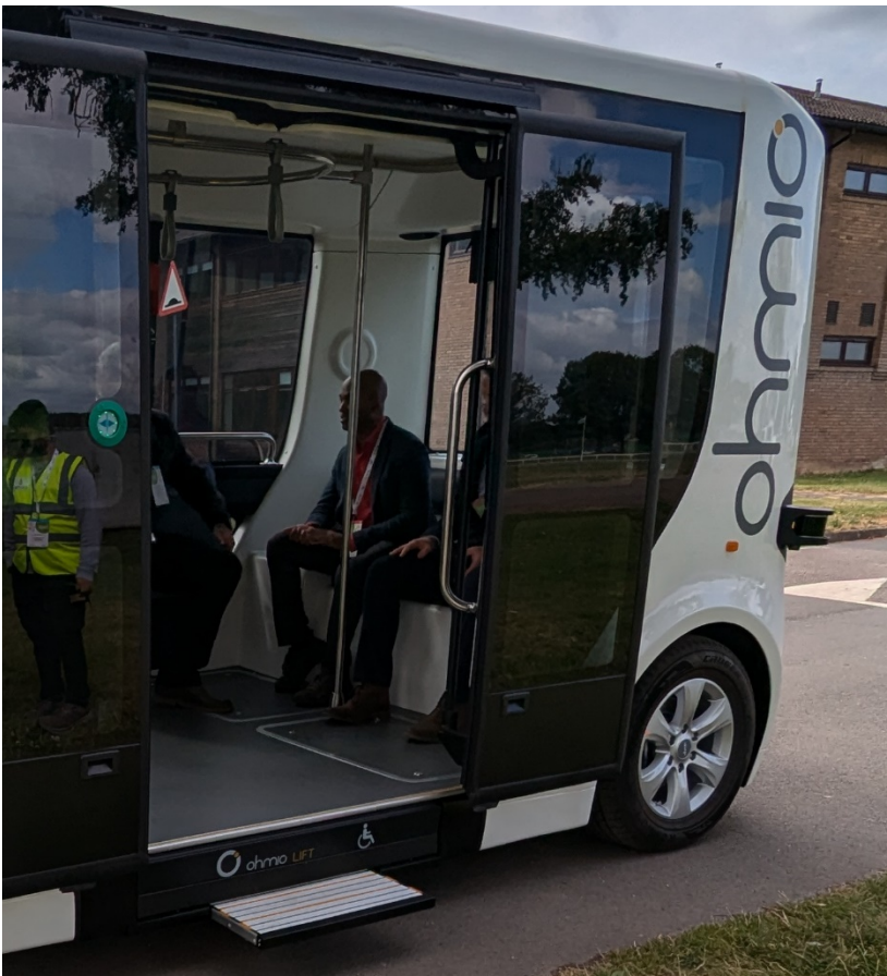
Figure 8: Ohmio (New Zealand based) Shuttle showing step / retractable wheelchair lift just under door 15
